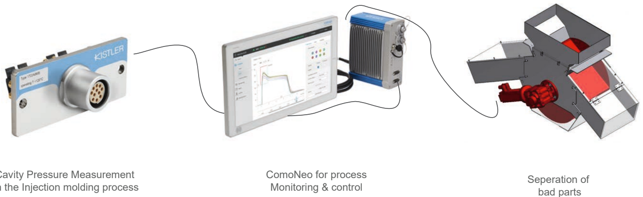
Figure 20: Structure of a monitoring system.
