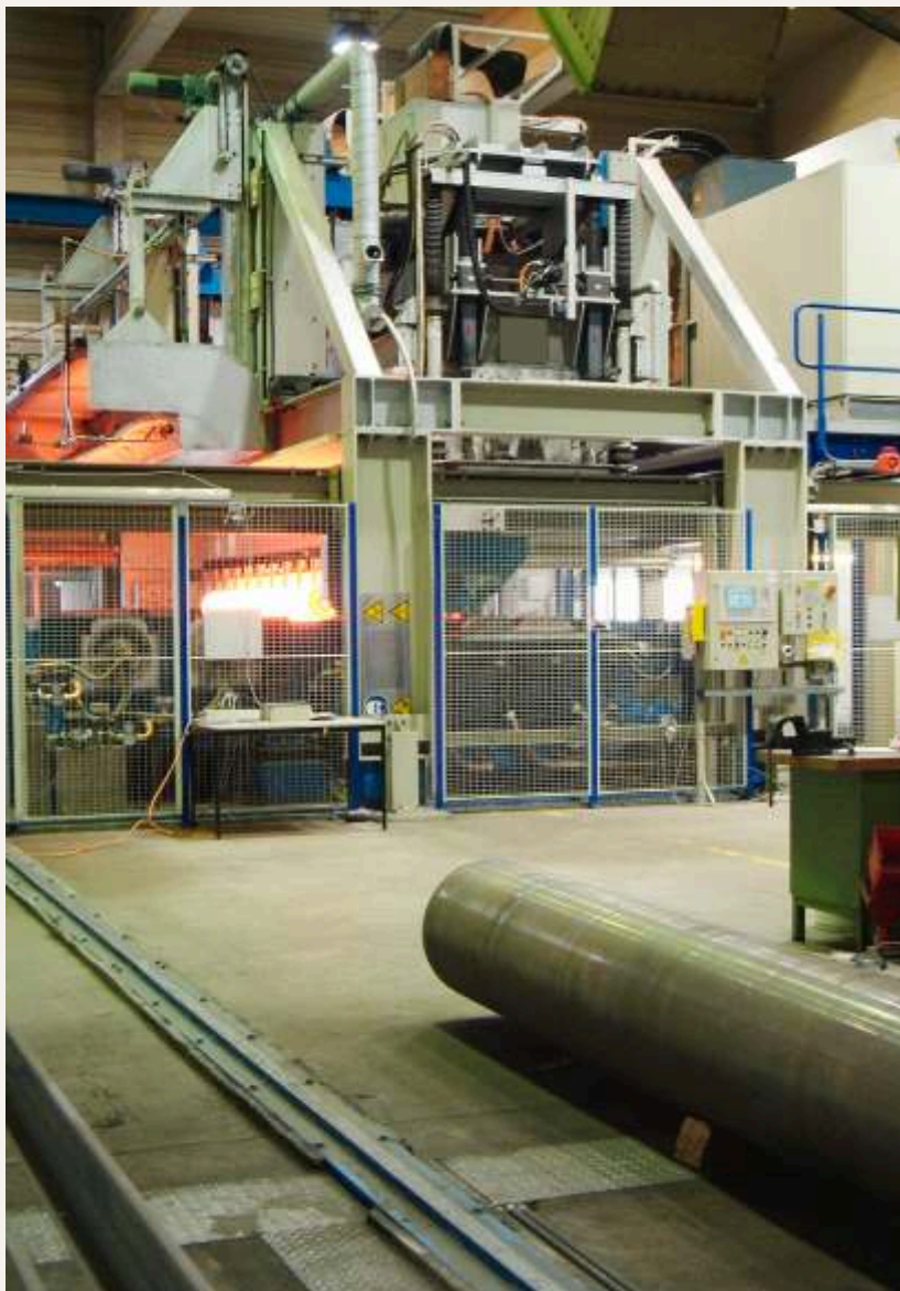
Centrifugal casting plant for large barrels of up to 8 tonnes
