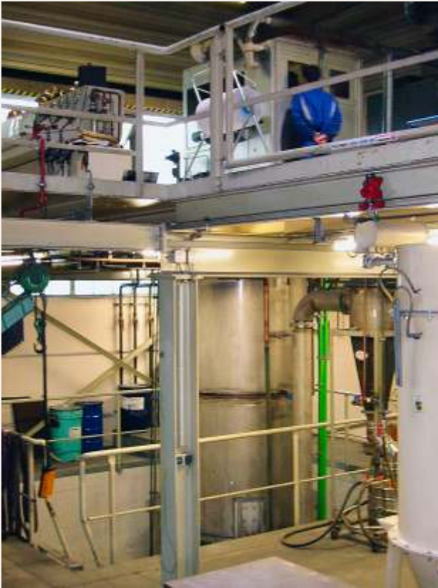
Gas atomisation plant for metal powder production
